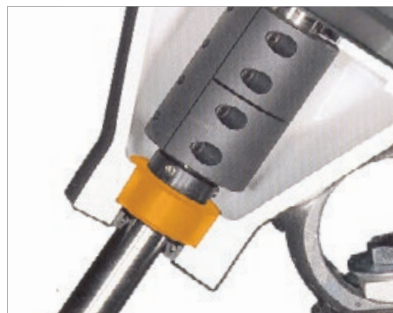
c Auxiliary bearing available with clamp mount (shown) and pedestal mount to limit overhung loads on drive.
